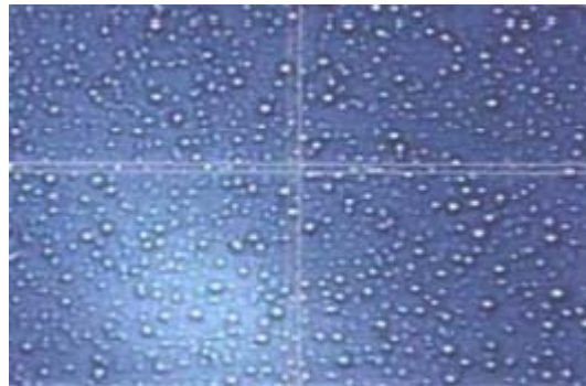
Figure 1. Photomicrograph of Water Particles in a Diesel Oil Emulsion
