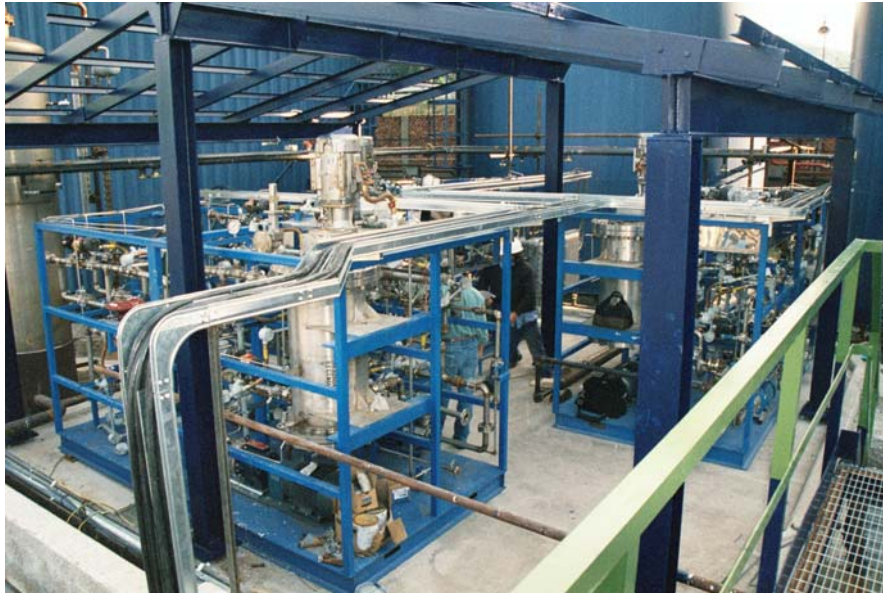
Figure 2a. Stationary Emulsified Fuel Blending Unit Located at Iplom Refinery, Busala, Italy
