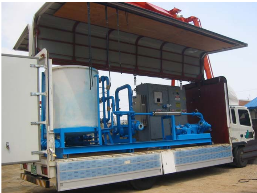
Figure 2b. Mobile Emulsified Fuel Blending Unit Located at Daesang Food Processing Plant, Ganchon, Korea
