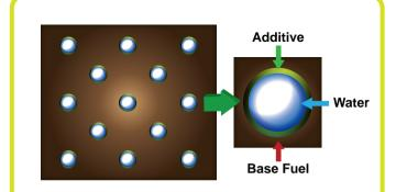
Oil-phase emulsified fuels are composed of microscopic droplets of water stably suspended in oil such as diesel fuel and fuel oil.
